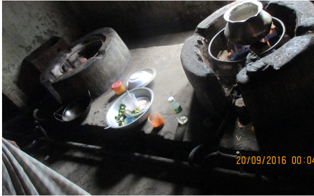
A burner being utilized inside the factory for cooking purposes. This is a dangerous practice and contrary to safety regulations, as it involves the use of open flames and non-compliant gas supplies.
